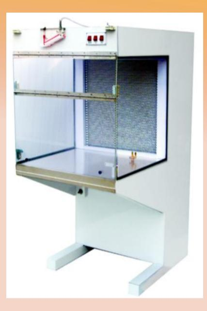
$\succ$  Its allowed to working for long period.  $\blacktriangleright$  Made up of stainless steel with no gaps or joint. PRINCIPLE – based on flow of current to create uniform velocity along parallel line, which helps in transforming microbial culture in aseptic condition to avoid the dust and contamination. ► Working - filter pad a fan and HEPA filter (
